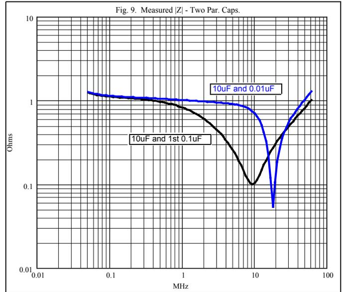
As might be expected, the 10 uF in parallel with the 0.1 uF provides the better decoupling over most of the frequency range.
