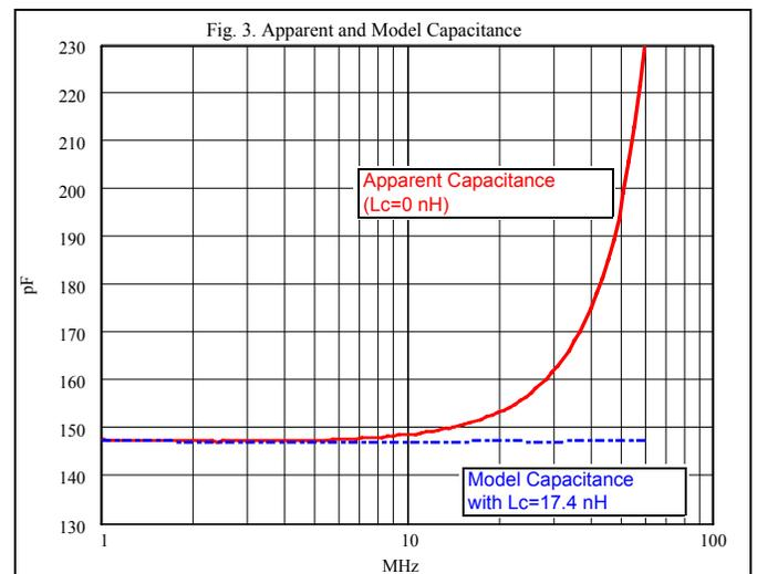
it clearly is not. The effect of series inductance is to lower the overall measured reactance at any given frequency and hence results in an apparent capacitance that increases with frequency.
