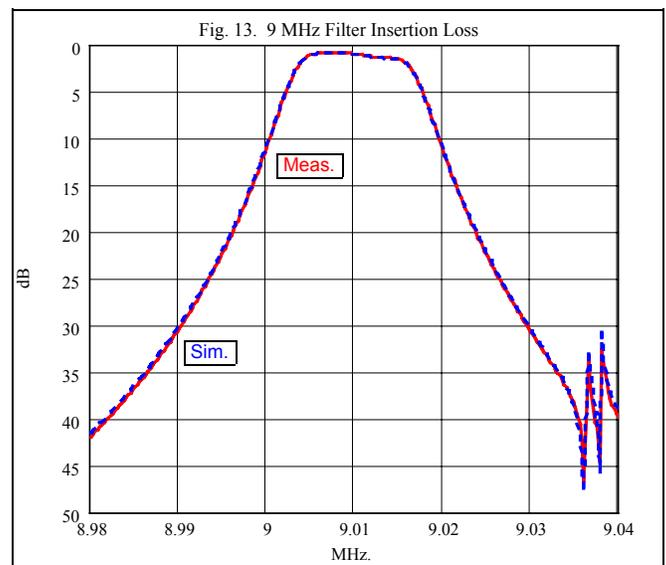
The correlation between measured and simulated insertion loss is quite good, even including the responses at the crystal spurs between 9.035 and 9.040 MHz.
