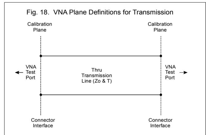
This VNA lends itself to a full *Open, Short, and Load* (OSL) calibration for reflection measurements and a modified *Response* calibration for transmission measurements. These
