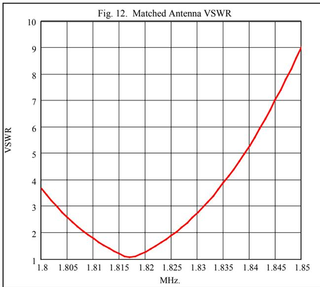
Clearly, a good impedance match has been obtained, quite close to the 1.82 MHz design point, without resorting to intentionally adjustable components. The 2:1 VSWR bandwidth is relatively low at about 18 kHz, which is typical for such relatively short antennas. Changing the spacing between turns on the larger inductor can also be used to move the minimum VSWR point to make this unit usable over the lower 40 kHz of this band which covers the author's interest here.
