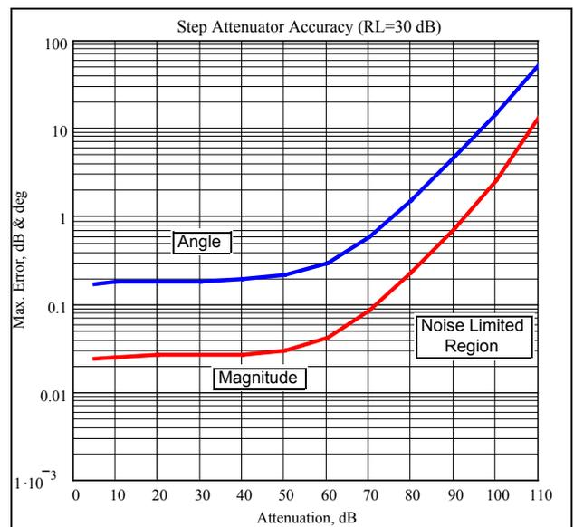
The errors seen here at 10 MHz will be larger at the 50 kHz and 60 MHz end frequency limits due to increased  $\Gamma_S$  as seen in the RF DDS return loss plot. However, the error at the end frequencies can be reduced with the addition on the source side of either external pads or a pre-amp with an attenuator at its output.
