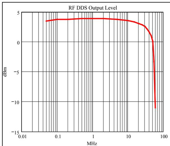
LO DDS filtered output (approx. 6 dB below RF DDS thru 30 MHz):
