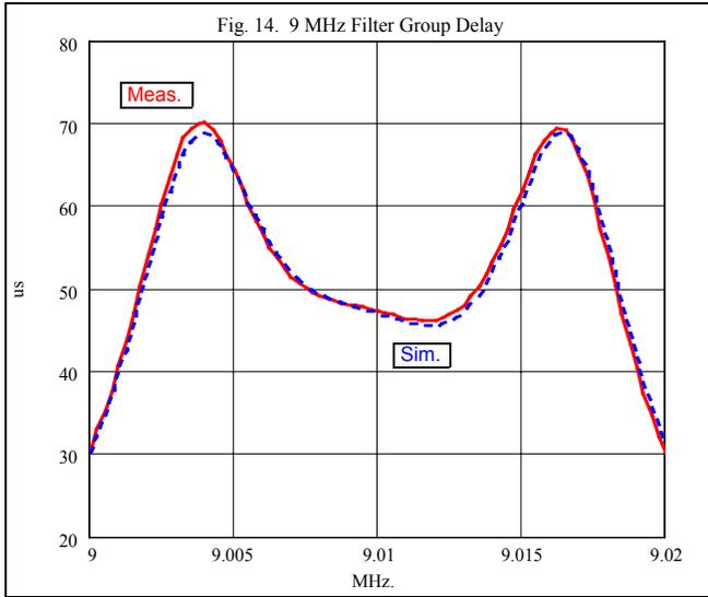
phase changes with frequency, is the more difficult of the two parameters to obtain accurately.
