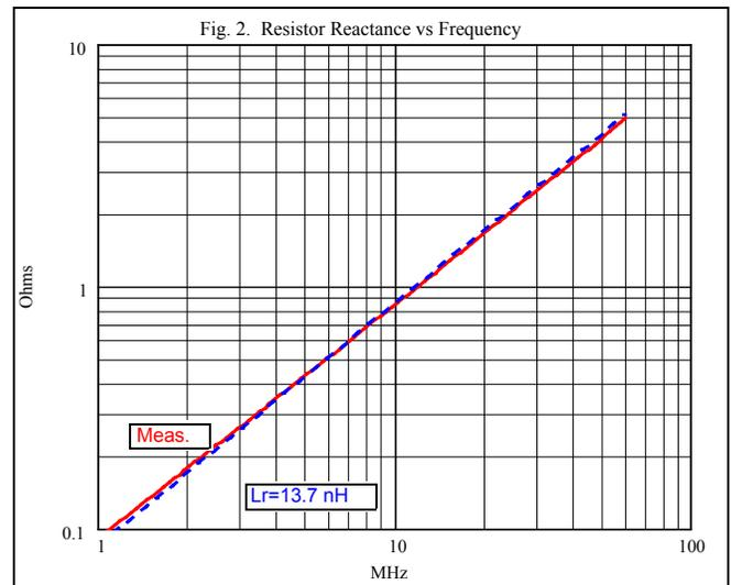
There is good correlation at 1 MHz between the resistance measured there and a 4-point Kelvin probe DC resistance measurement. There appears to be skin effect and proximity effect dependencies of resistance with frequency. Note however that the total change in resistance is only 130 milliohms.
