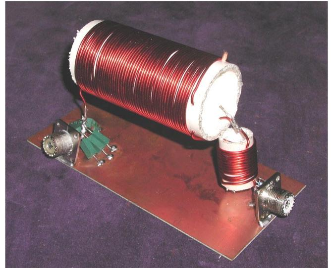
Since there were some differences between the desired or estimated and the measured values, the MathCAD program was used to re-check the match using the measured and new estimated values. The predicted match was still good with  $\text{VSWR}=1.13$  and  $\text{return loss}=24 \text{ dB}$  at 1.82 MHz.
