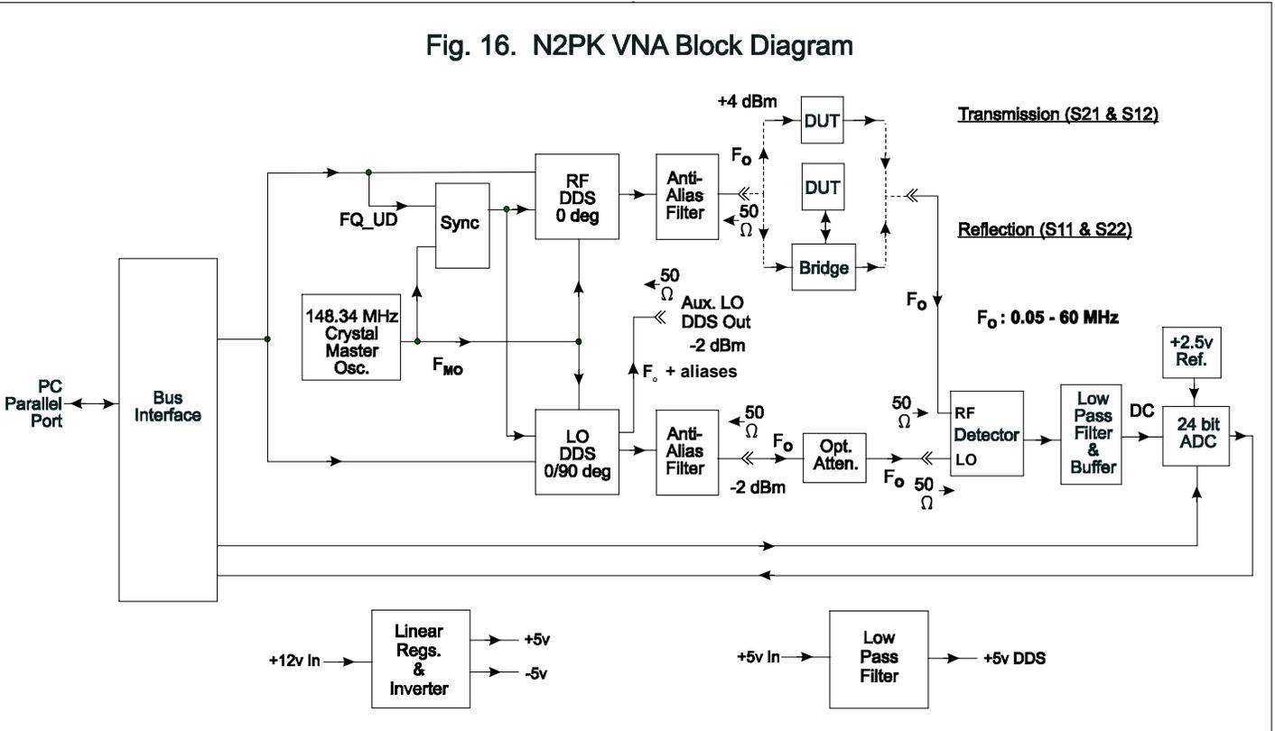
The Detector is a balanced mixer (see later) and the LO DDS provides the reference phase signal to the LO input of the Detector.
