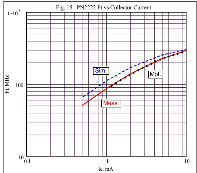
The correlation between the measured and the Motorola data is particularly striking. Normally there's a peak in F<sub>t</sub>, but apparently the collector currents used weren't high enough for that to occur. The Motorola datasheet indicates that peak occurs at I<sub>c</sub>=25 mA in this transistor.
