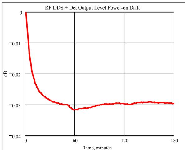
b) Detector offset voltage power-on drift:
