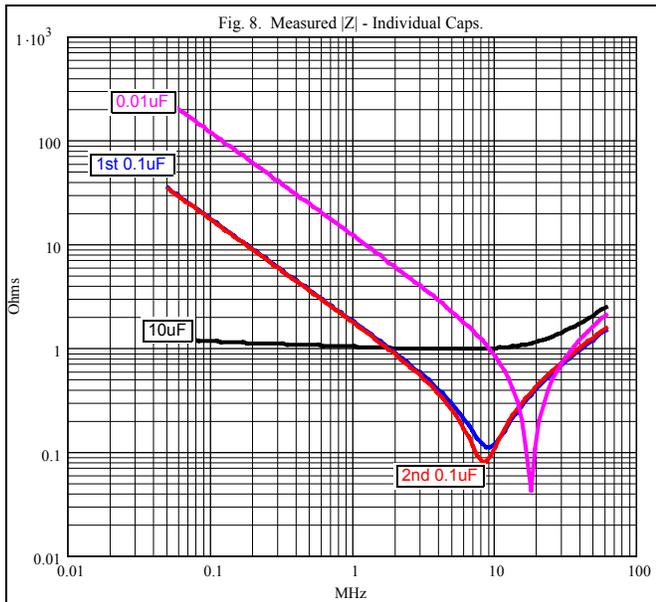
Due to the dominant effect on |Z| of Rs for the 10 uF capacitor over most of the plotted frequency range, the file data for Cs at 50 kHz and Ls at 60 MHz was used.
