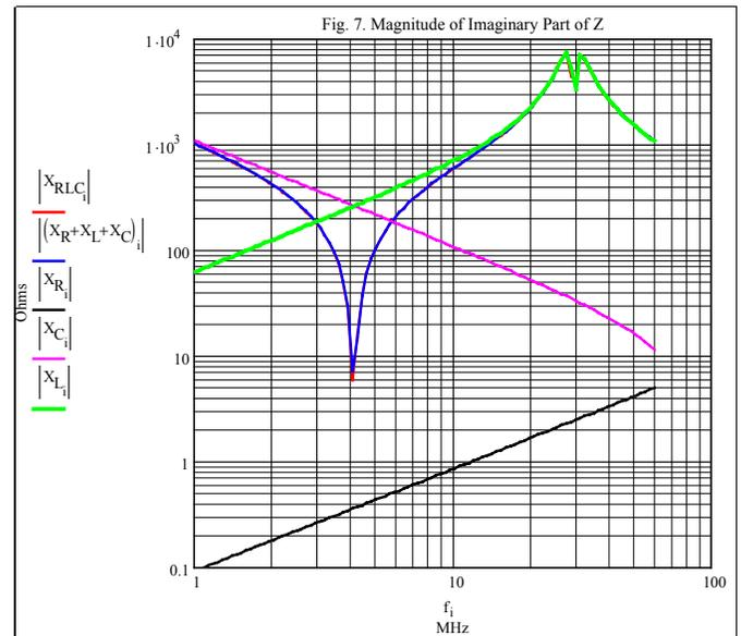
The observed series resonance is at 4.126 MHz vs. the calculated resonance at 4.135 MHz for the individually modeled components.
