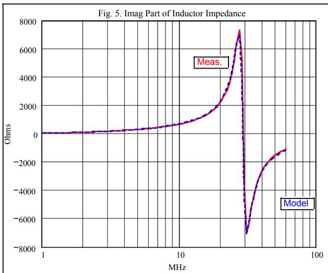
The model for the inductor is consistent with measured data over most of the 1-60 MHz range, including well above the parallel resonance at 29 MHz. Below 2 MHz, there is an increasing error in the real part of Z.
